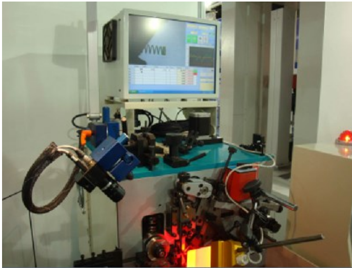
CAMERA CONTROL 100% Testing of Length and Spring Diameter
